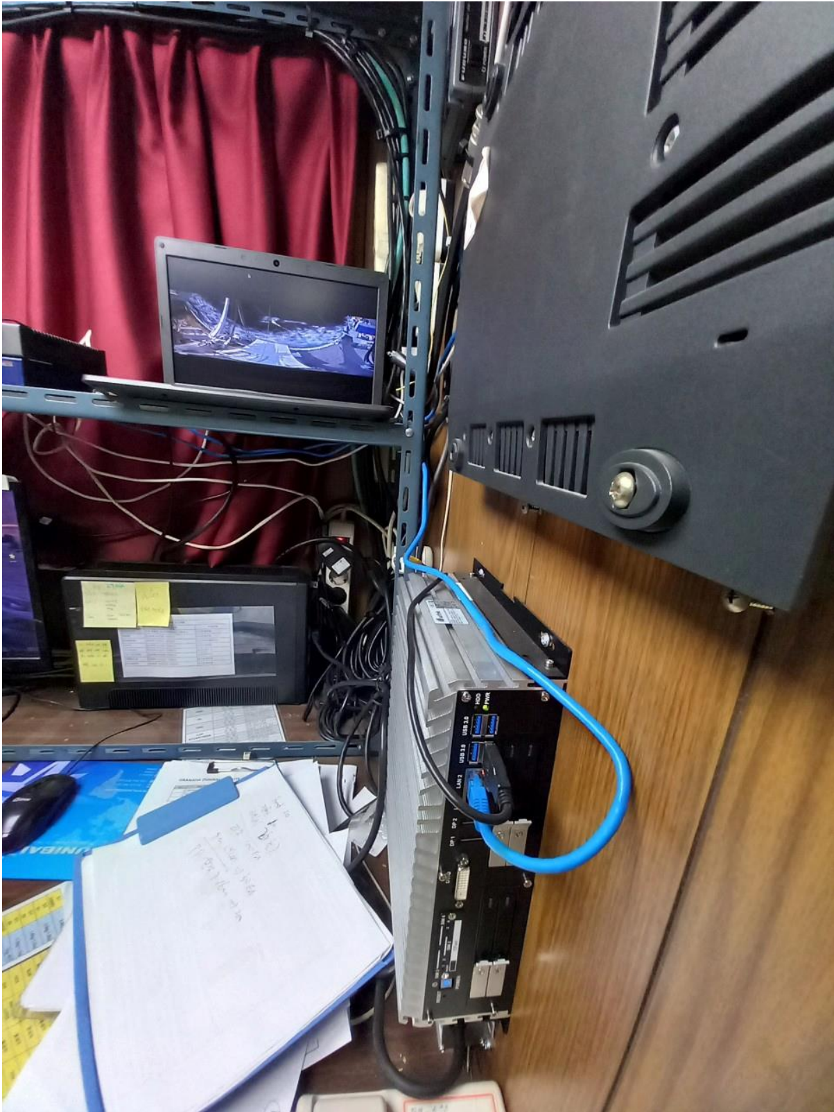
Figure 5: Photo of the computer and hardware system that is powering the cameras installed onboard the vessels within the FIP fleet.
