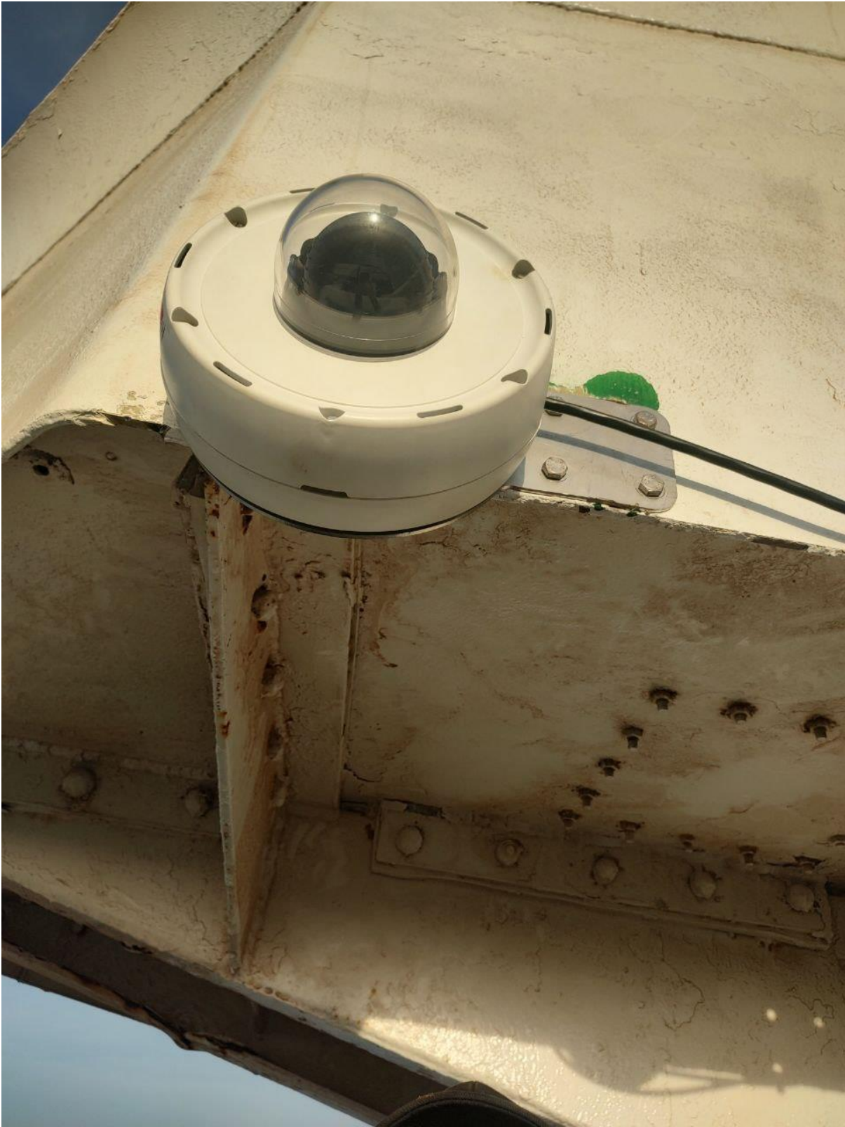
Figure 4: Photo of a camera installed on one of the vessels in the Capsen and Grand Bleu FIP fleet
