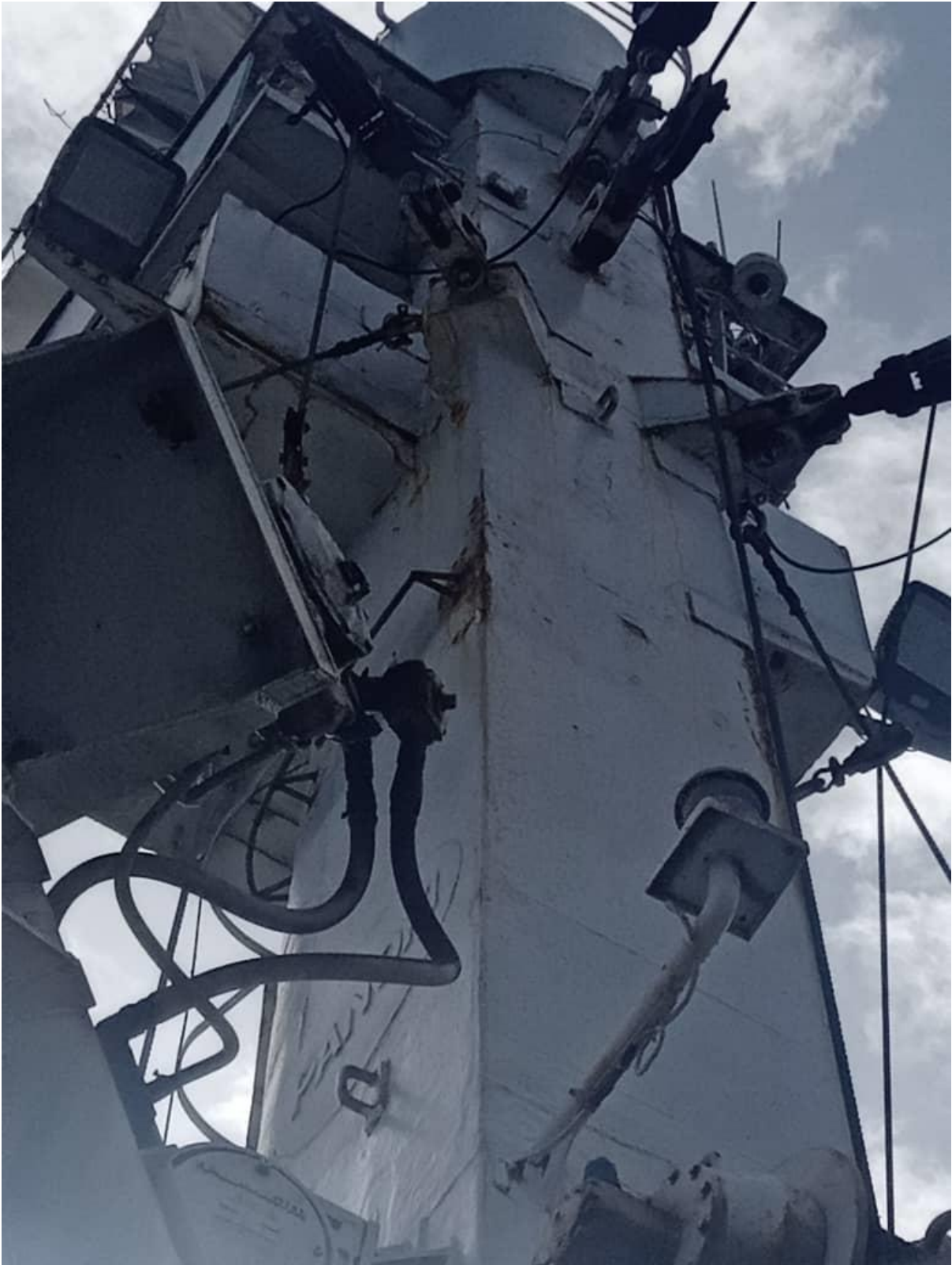
Figure 2: Photo of the EM camera positioned on the mast of the vessel to capture on-deck activity
