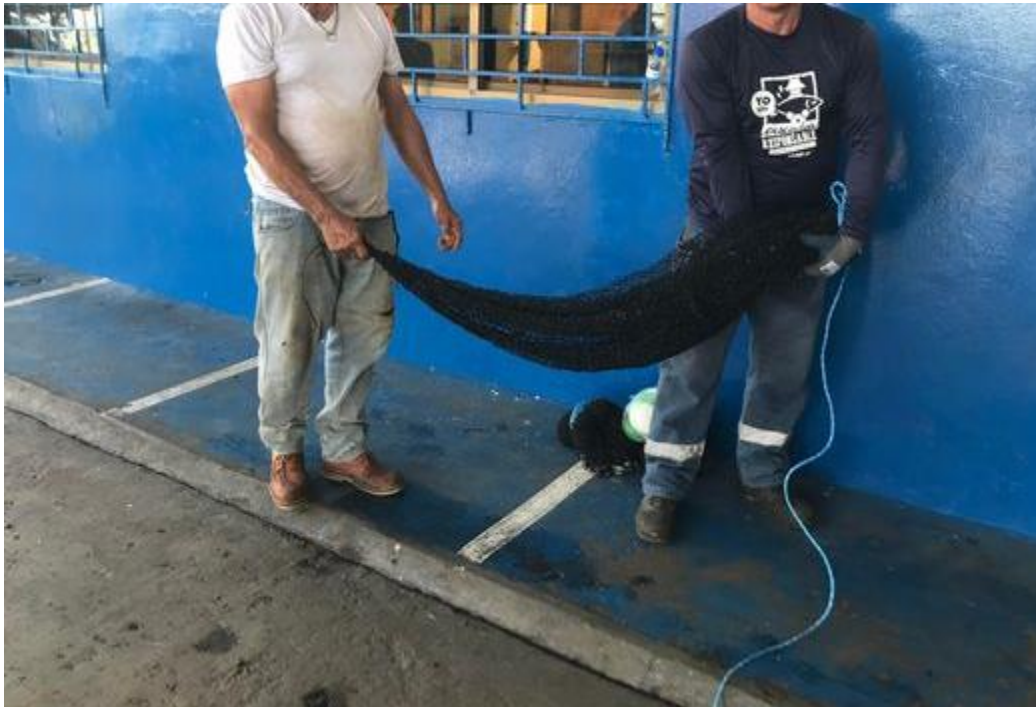
Figure 2: Photo of the sling net used to bring hooked ETP species, including sharks and turtles, onboard the vessel for safe and efficient hook removal
