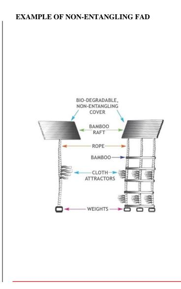
1. The surface structure of the FAD shall not be covered, or only covered with non-meshed material If a sub-surface component is used, it shall not be made from netting but from non-meshed materials such as ropes or canvas sheets.
