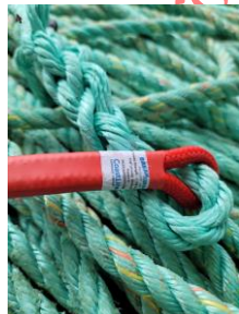
Figure 13: One of the three BreakAway release links attached to the 75-fa HydroPro-Polysteel buoy line
