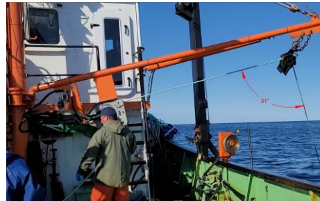
Figure 11: Included angle of two strings of the 5/8" traditional buoyline around the directional pulley
