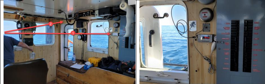
Figure 5: Tensiometer display meter is not aligned with the line of sight #1 of the operator
