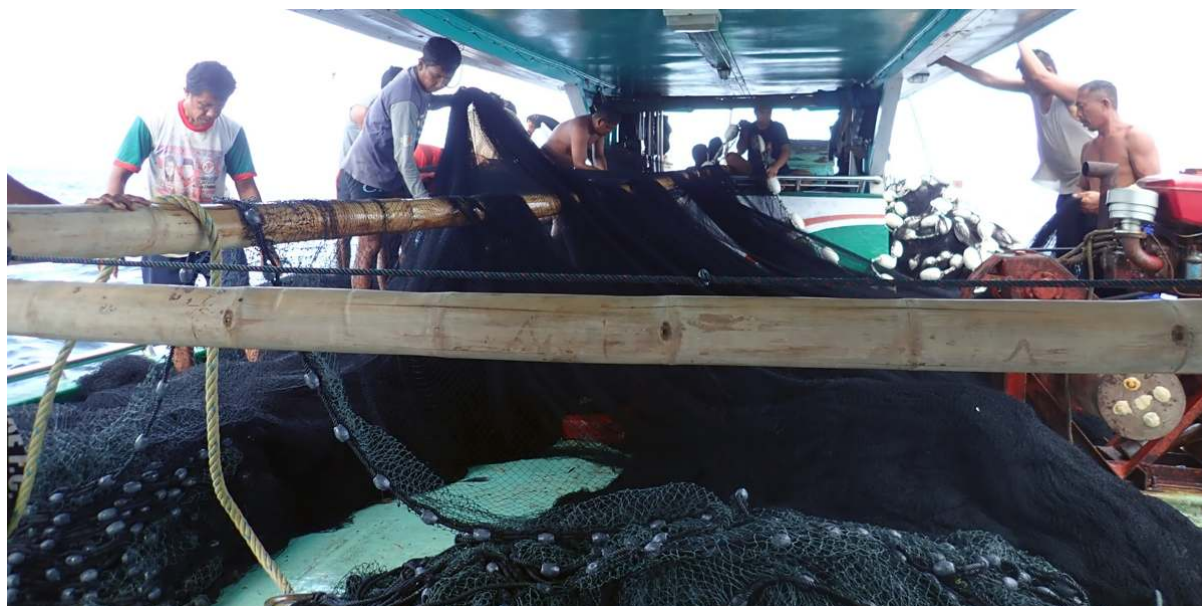
Figure 1.4: Purse seine, typical for IAW. Most of the purse seines used in Indonesia are small, only a fraction of the size of those deployed from industrial purse seiners operating on the high seas.
