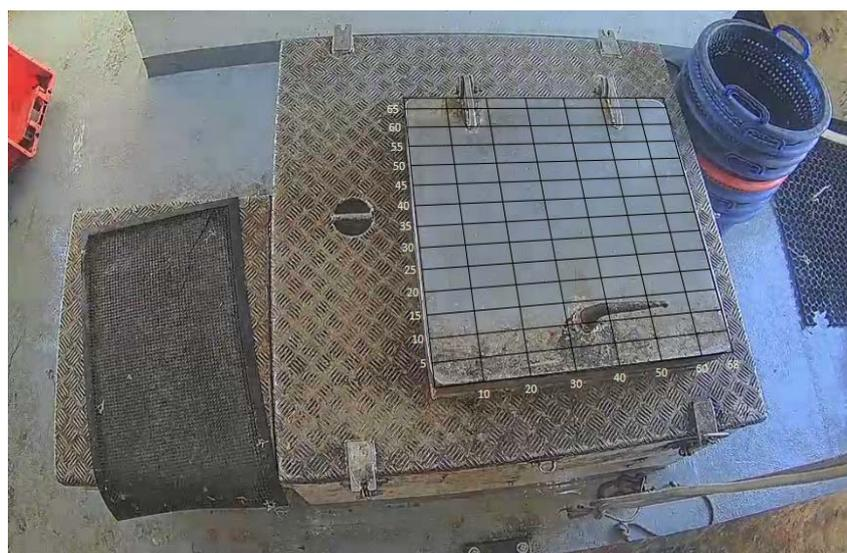
**Figure 2.** Example of a calibrated hatch onboard a commercial fishing vessel. These areas will vary from vessel to vessel, depending on available surfaces and the species being measured. This image is provided as an example from a non-tuna fishery. For tuna and tuna-like fisheries, the defined areas will have to be larger to accommodate larger species (image source: Centre for Environment Fisheries and Aquaculture Science - CEFAS).
