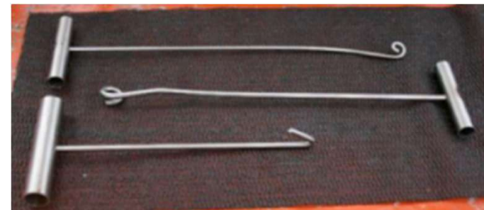
Pigtail and J type dehookers (Photo: M Parga SUBMON)
