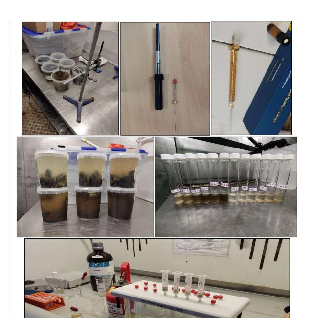
**Figure 1.** PDMS fibre deployment and SPME holder (top left and top middle). Glass syringe used for DI (top right). Soaking containers with green crab and mussel material stacked above (middle left). Samples collected in universal glass containers for SPE filtration prior to analysis (middle right). SPE filtration set up, with SPE cartridge filled with water sample, drawn down through apparatus using vacuum.
