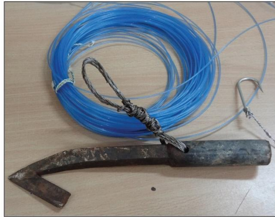
Image 7: Longlines and hooks used for catching sharks in Thoothoor
