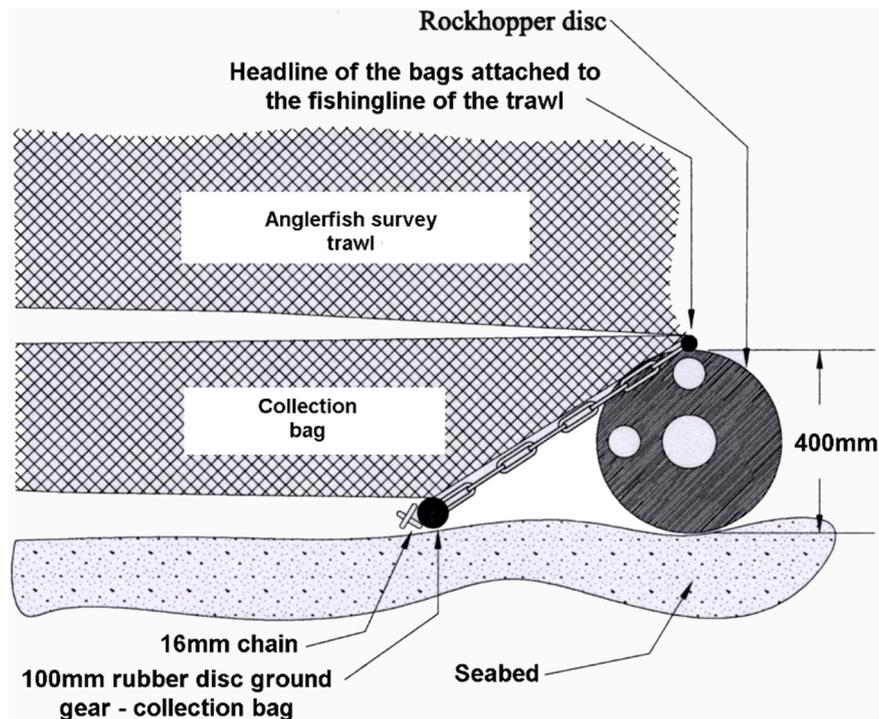
Fig. 2. Side elevation of the trawl used in the 2006 and 2007 anglerfish (*Lophius piscatorius* and *L. budegassa*) gear selectivity trials, showing the mouth of the collection bag and lower part of the main survey trawl.
