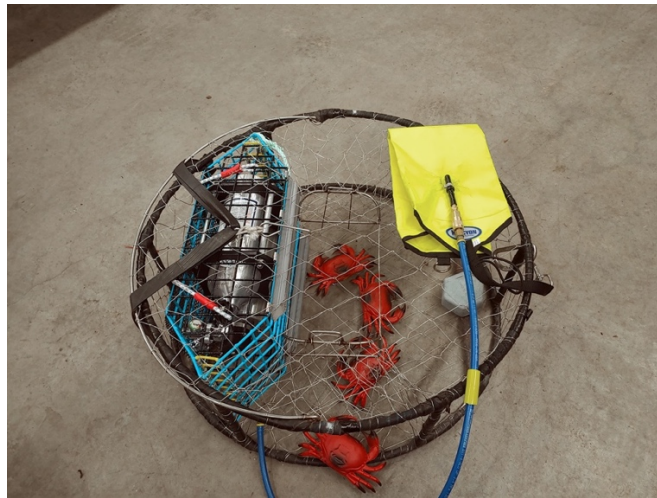
Figure 6. A SMELTS crab raft wireless trap with the bag uninflated.
