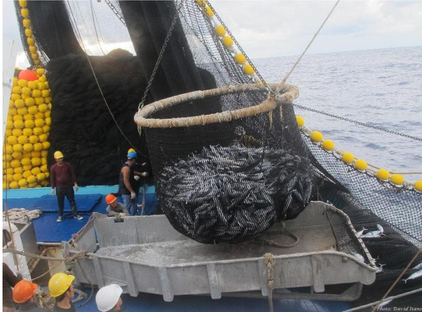
**Figure 7.** The use of the hopper in a purse seiner vessel fishing tropical tuna
