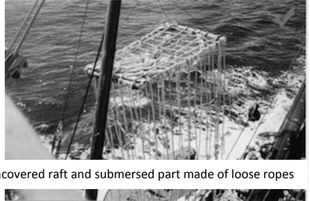
**Fig 6.** Device with uncovered raft and submersed part made of loose ropes
