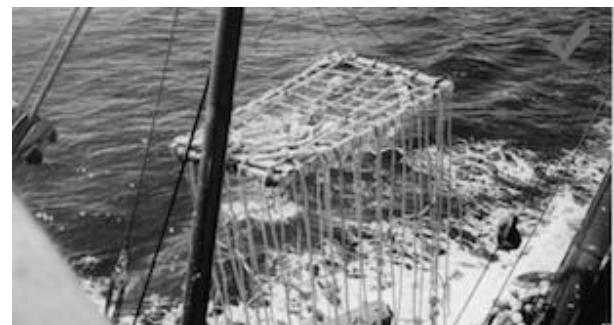
**Fig 6.**Device with uncovered raft and submersed part made of loose ropes
