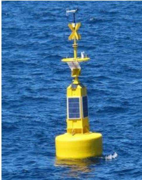
Equipped with oceanographic sensors for continuous collection of observations of **waves, current, water temperature, water salinity, water turbidity, water dissolved oxygen, fluorescence, PH, ...** from the Dakhla area.
