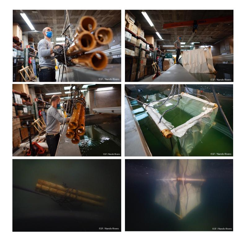
**Figure 4**. Assessment of the evolution of the density of the organic materials (bamboo canes, rope and cotton fabric and cubic structure) during two months in a seawater tank.
