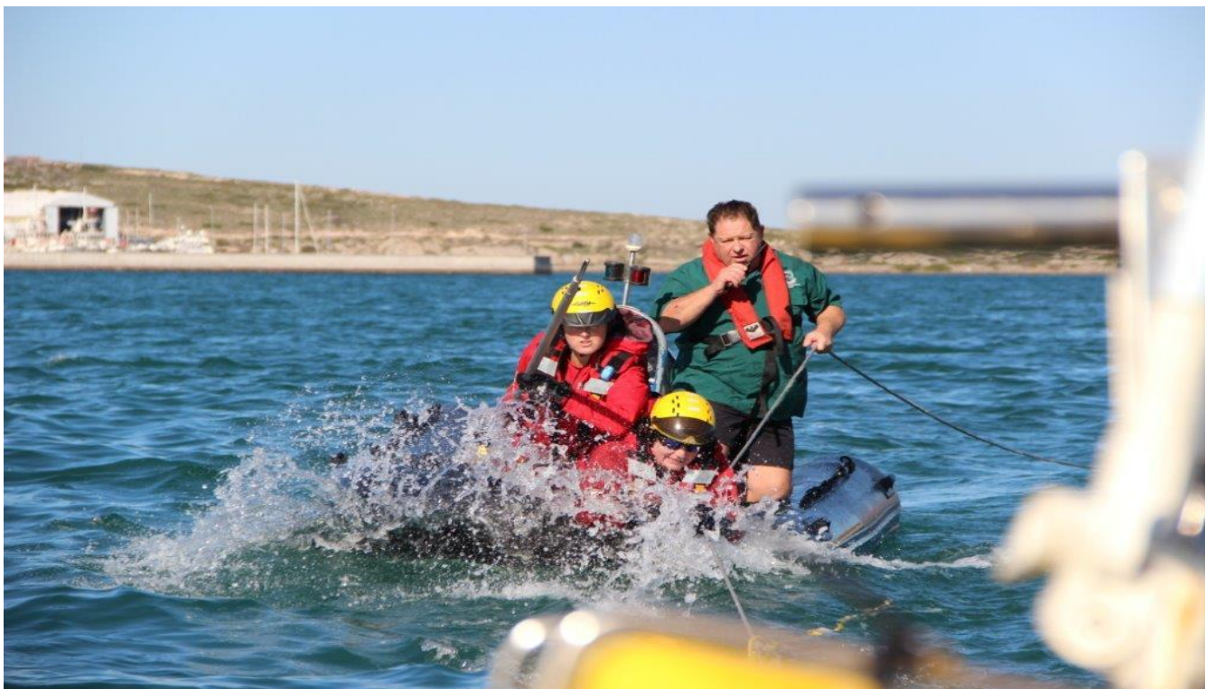
Figure 13: Pulling the small vessel up the control line towards the “whale” and reporting progress to mother vessel:
