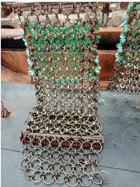
Figure 11 Right; skids attached to dredge bellies used in the LISIG project compared with left standard Newhaven bellies.
