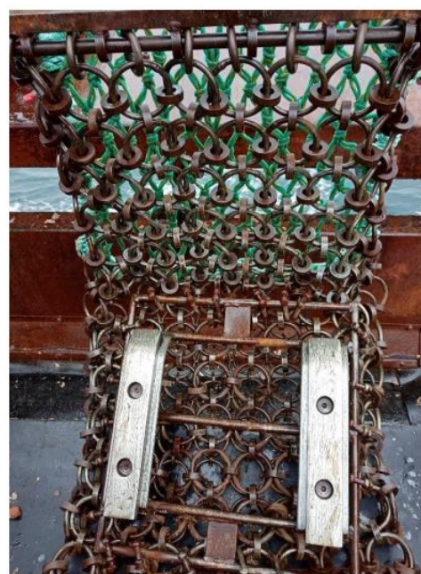
Figure 11 Right; skids attached to dredge bellies used in the LISIG project compared with left standard Newhaven bellies.
