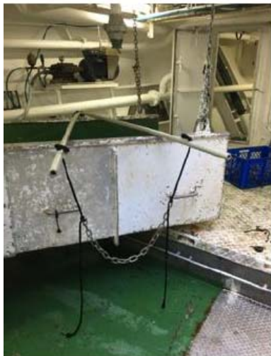
Figure 2. Stretcher configuration prior to adding the netting (left) and use at sea (right).
