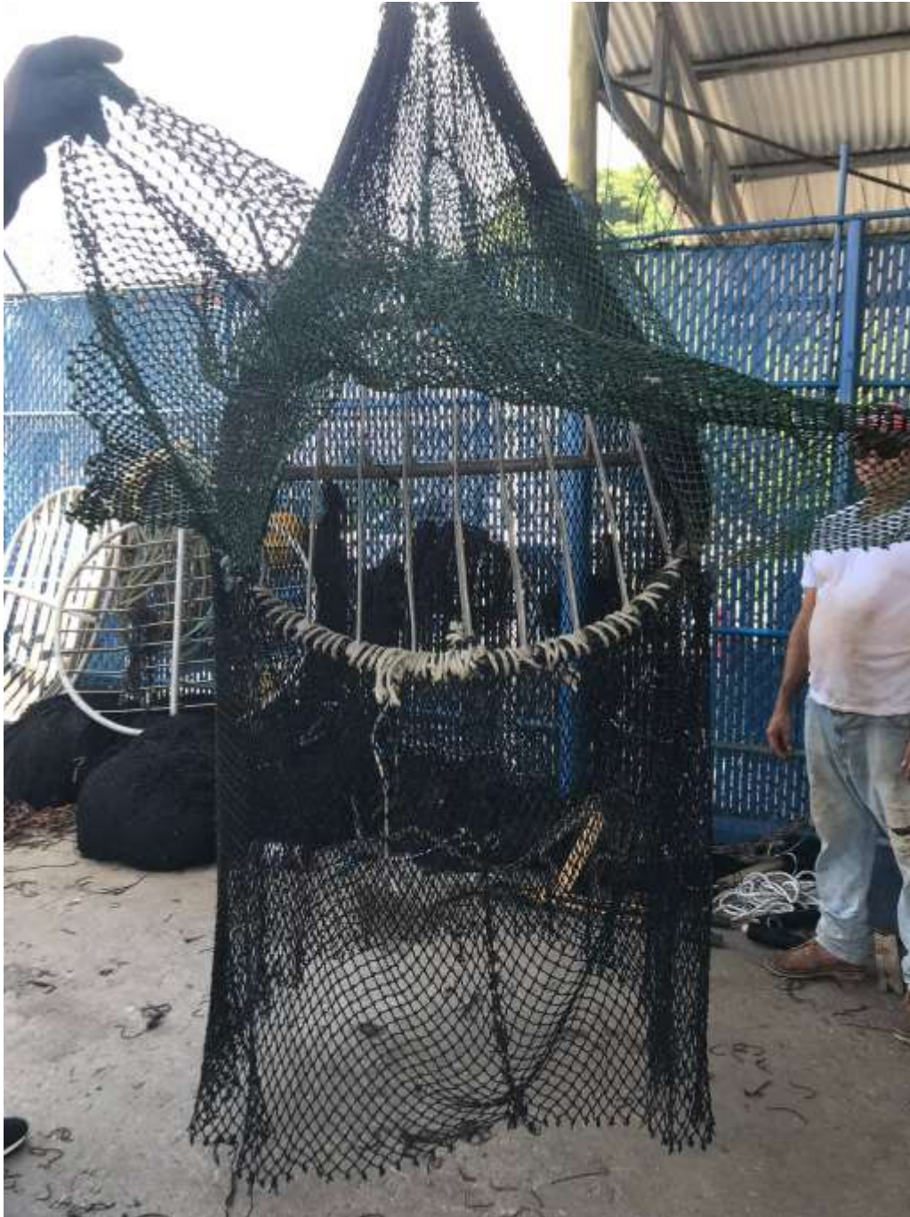
Figure 2: Photo of a TED on part of the bottom trawl net used by the FIP taken during a site visit to Panama in 2022
