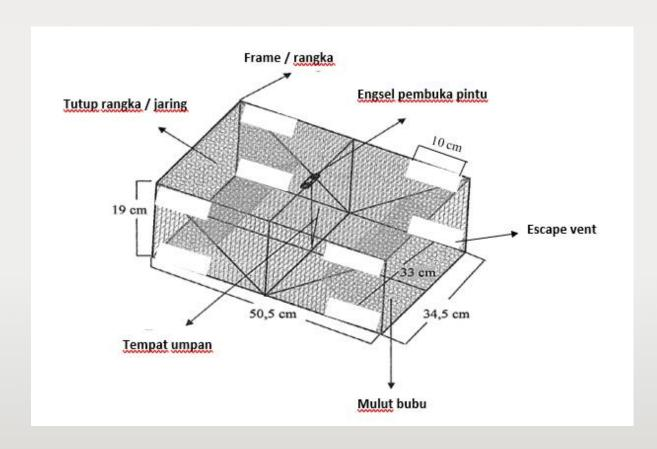
Folding trap consists of a frame made of iron and a net. The escape vent modification shown in the picture is made at the ends on both sides with a width of 10 cm and a height of 3.5 cm. So there are a total of eight escape vents that are expected to be able to escape crabs under 10 cm. A total of 40 folding traps with escape vents were made and made in Jepara, Central Java.
