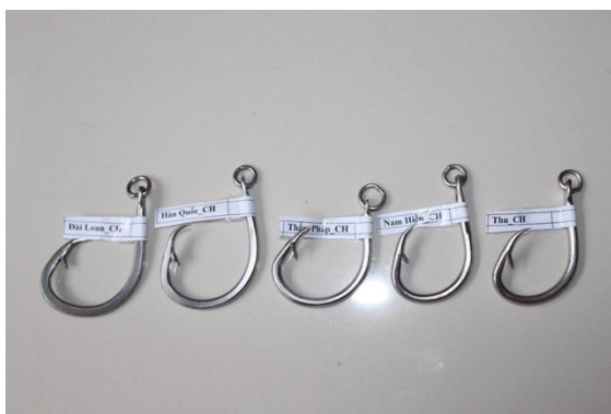
Figure 8. Five types of C-hooks in Vietnam tuna fisheries
