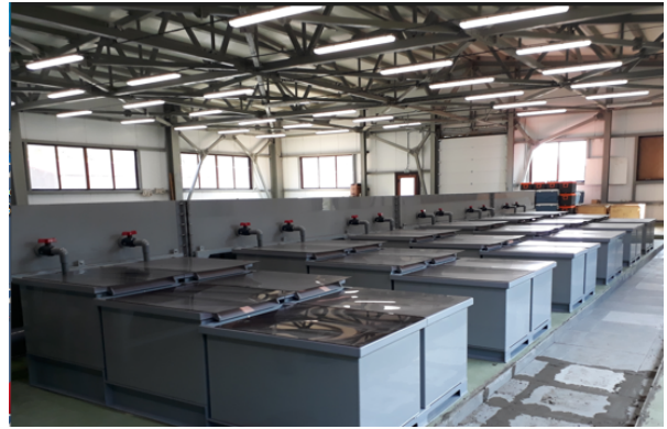
Figure 6. A workshop with Japanese-made "Box" type incubation machines
