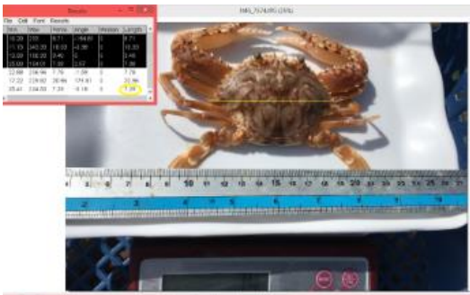
Figure 3. Measurement of crab carapace width
