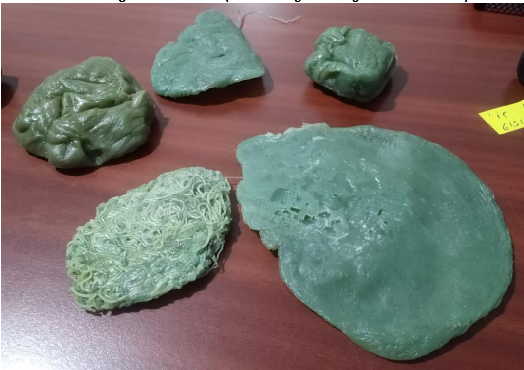
13.- Panel tests for roofing made with nets (Melt testing of fishing nets in reused oil)
