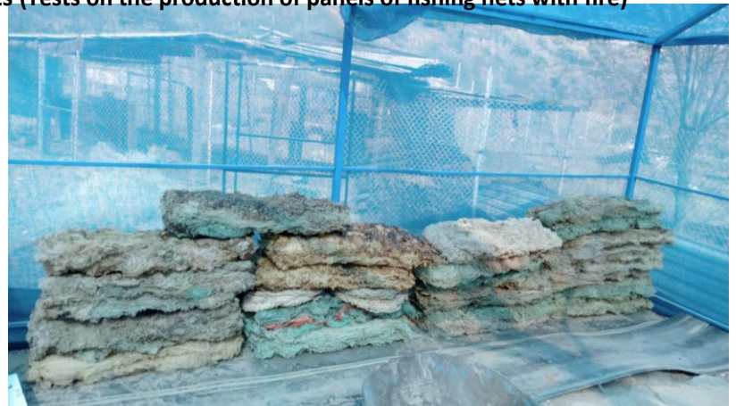
12.- Panel tests for roofing made with nets (Tests on the production of panels of fishing nets with fire)
