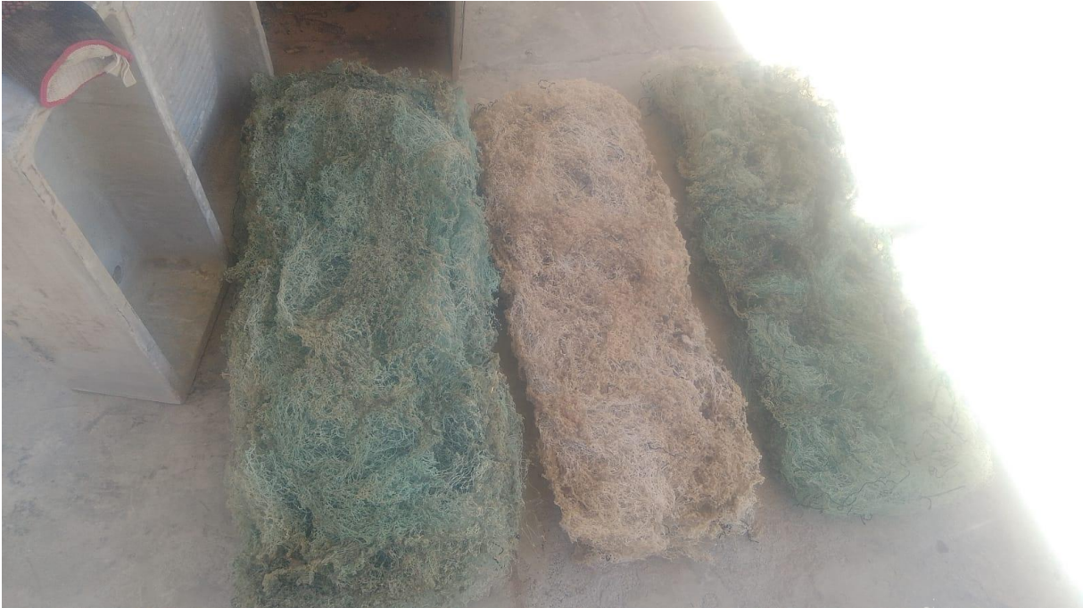
13.- Panel tests for roofing made with nets (Melt testing of fishing nets in reused oil)
