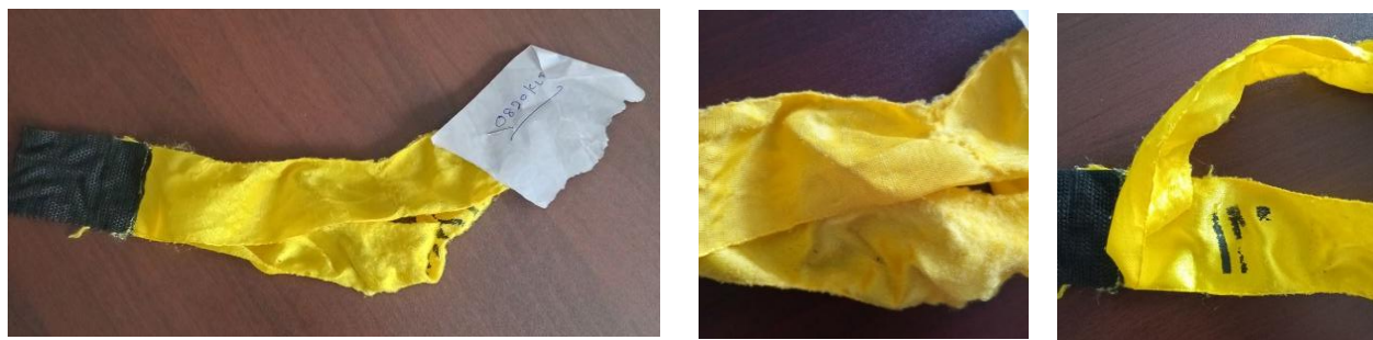
Figure 3: The material of the cloth tag was crushed and damaged, the print is totally gone away
