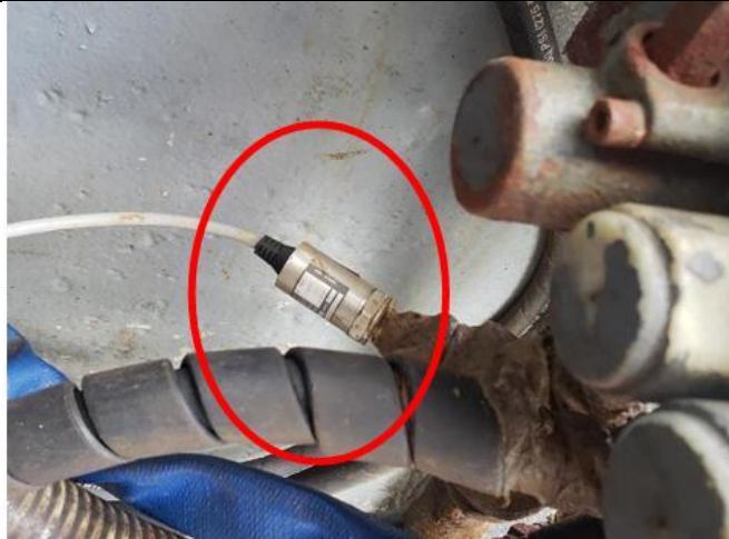
Example of installed hydraulic sensor (Mouser M5241)
